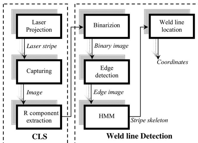
Fig. 1 Flowchart of the proposed CSL based weld line detection approach.
