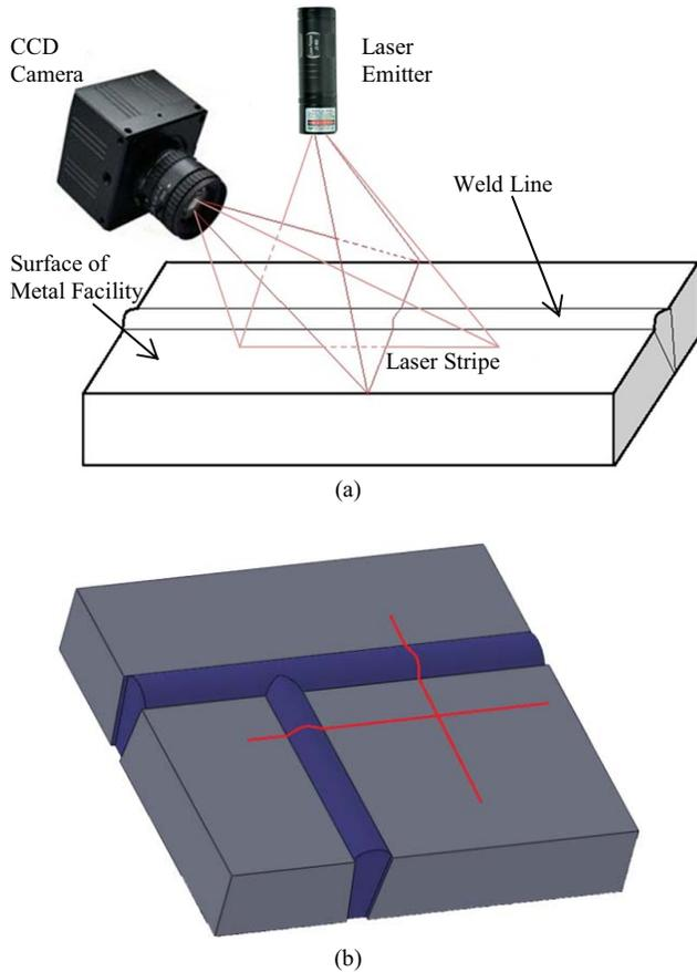
Fig.2 (a) Illustration of CSL platform. (b) illustration of laser stripes on a weldment surface of a cross weld line.
