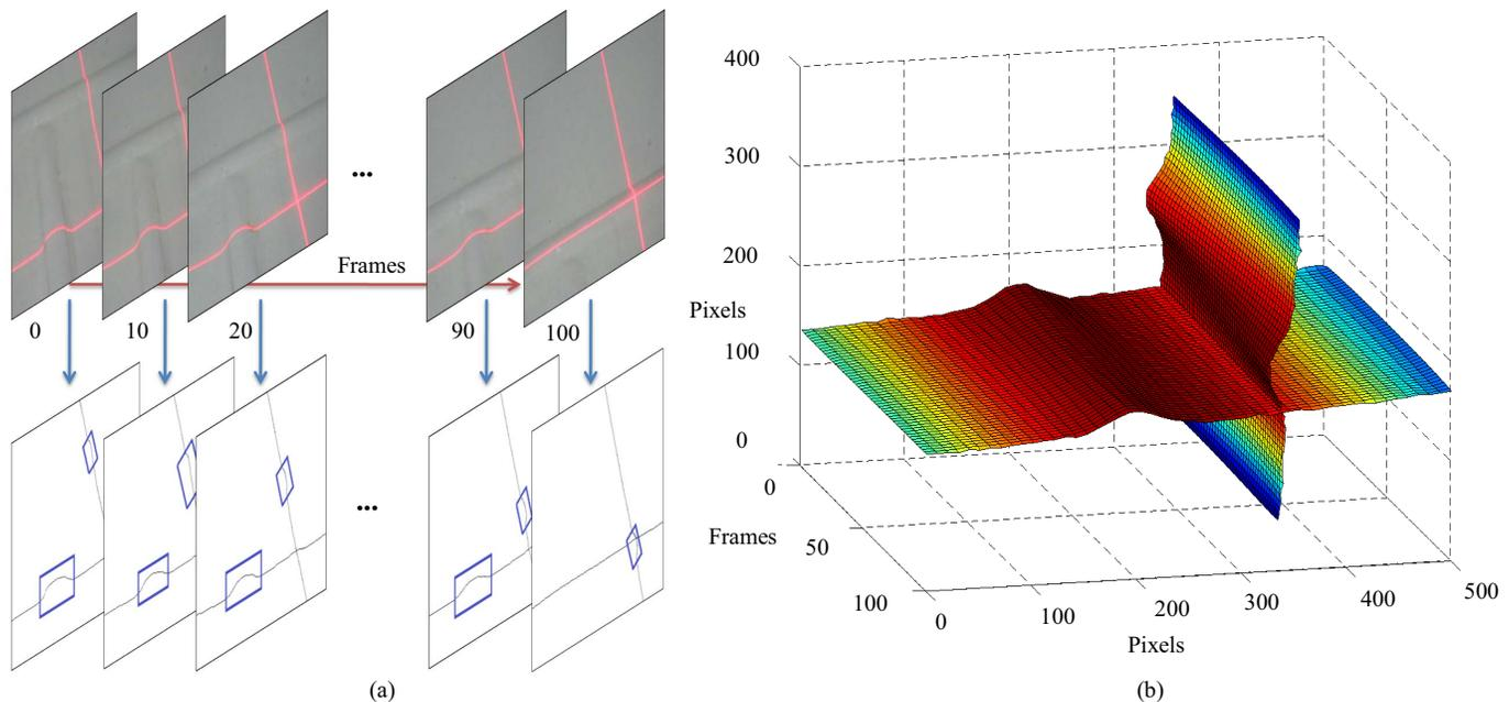
Fig.8. (a) From left to right, images are captured when the platform is moving close to a weld line intersection. (b) shows the weld locations in successive video frames
