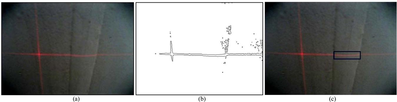
Fig.3 Extraction of edge image and filtering the stripe edges with an HMM. (a) A captured laser stripe image, (b) Canny edge image, (c) A weld line location on laser stripe
