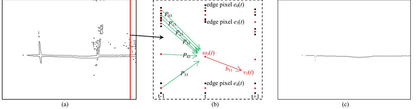
Fig.4 HMM for stripe detection. (a) Edge image, and (b) illustration of steps of HMM, the states are from three columns of edge pixels of (a), where black points represent edge pixels, and red points represent midpoints of adjacent edge pairs. (c) Detected stripe skeleton.
