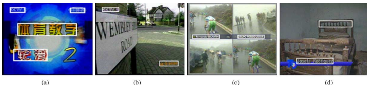
Fig. 14. Images with failures and false alarms. (a–c) Examples containing missed text and (d) contains a false alarm.
