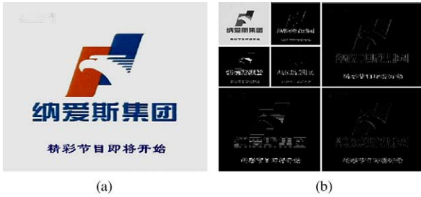
Fig. 2. Two-level wavelet transformation. (a) The original image with text in different font-size and (b) the wavelet transformation images in two levels.
