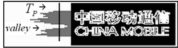
Fig. 6. An example of horizontal projection profile. Multi-line text can be separated at the ‘valley’ of the project profile.
